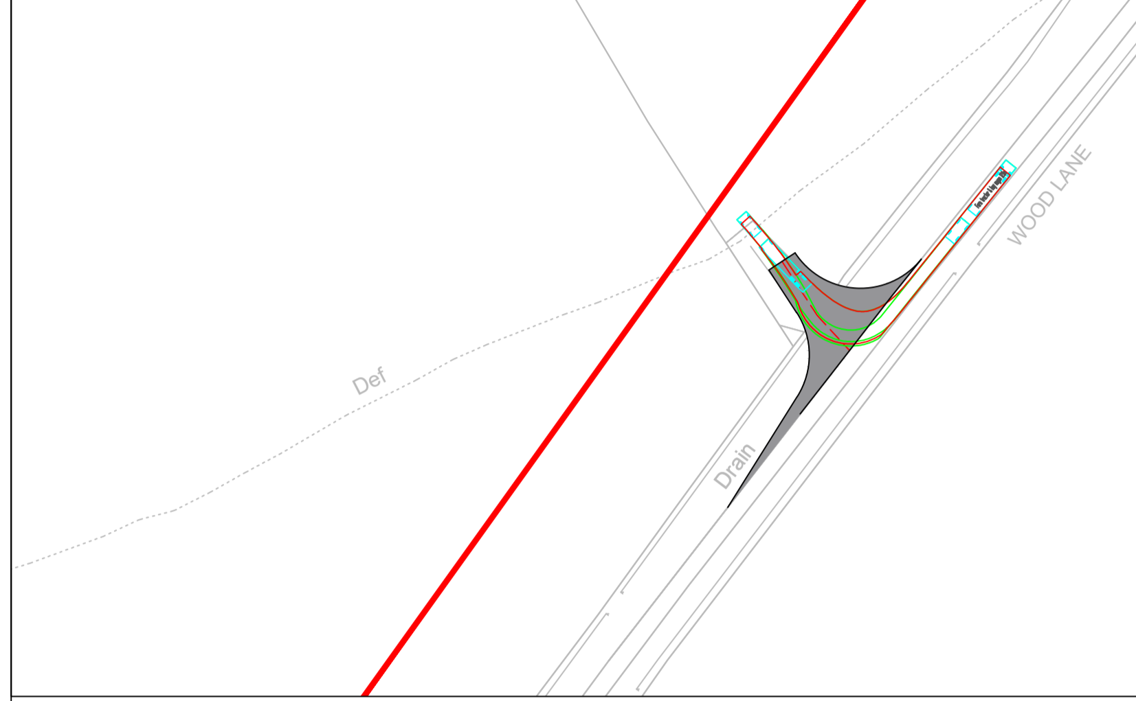
INSET B: TRACTOR & HAY WAGON MANOEUVRE HEADING NORTH ON WOOD LANE, LEFT TURN INTO ACCESS - SCALE 1:1000
