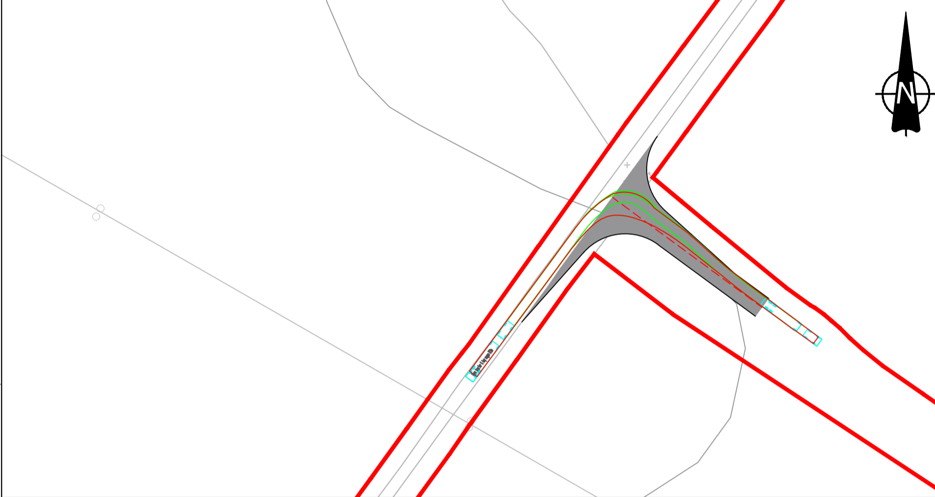
INSET B: TRACTOR & HAY WAGON MANOEUVRE HEADING SOUTH ON ROWLANDHALL LANE, LEFT TURN INTO ACCESS - SCALE 1:1000
